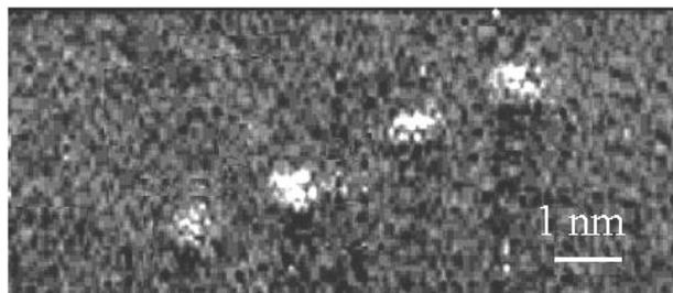
**Figure 2.** A typical STM image of a recorded pattern formed by a voltage pulse of 3.5 V applied for 5 ms; scanning conditions:  $V_b = 0.39$  V;  $I_t = 0.21$  nA.
