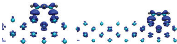
Figure 4. Electronic charge accumulation for B2 position along the [001] direction in a 3 \times 4 unit cell (left) and in a 6 \times 6 (right). It can be observed how in the 6 \times 6 the charge overlap between benzene and copper increases.
