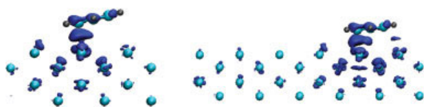
Figure 3. Electronic charge accumulation for B5 position along the [001] direction in a 3 \times 4 unit cell (left) and in a 6 \times 6 (right). The visualized isosurface value is 2.5 \times 10^{-6} \text{ e}\text{\AA}^{-3} and 8.2 \times 10^{-7} \text{ e}\text{\AA}^{-3} , respectively. In the 3 \times 4 unit cell the bonding occurs exclusively between the two closest copper atoms and the lowest carbon atoms. In a 6 \times 6 the bonding involves both sides of the benzene ring. Consequently the tilt angle decreases.
