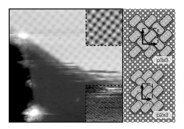
FIG. 2. Left: nc-AFM topography (raw data) of a monolayer island showing molecular and atomic scale resolution on the overlayer and substrate with insets adjusted for contrast ( $\Delta f = -8.7$  Hz, size: 20 nm, z scale = 5.5 Å). Right: schematic of proposed  $p3 \times 3$  monolayer epitaxy (top) and proposed  $p2 \times 3$  multilayer interface structure (bottom).
