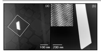
FIG. 4. (a) A tall crystalline island surrounded by a depletion region (indicated by the dashed box) caused by substrate induced dewetting ( $\Delta f = -8.4$  Hz, z scale: 3.6 nm). (b) PTCDA island after annealing ( $\Delta f = -2.3$  Hz, z scale = 7 nm). Inset: molecular resolution of the herringbone structure observed on top of the island ( $\Delta f = -25.5$  Hz, size: 15 nm, z scale = 0.1 Å).
