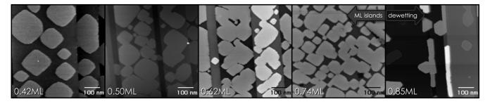
FIG. 1. Overview images ( $600 \times 600$  nm) of different submonolayer coverages of PTCDA on NaCl. At 0.74 ML and below, only monolayer islands are observed, at 0.85 ML, monolayer islands and tall crystalline islands coexist.
