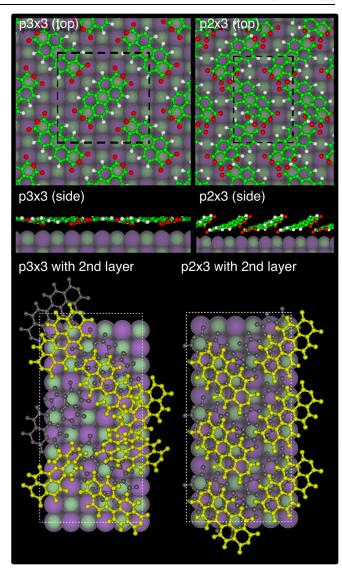
FIG. 3 (color online). Top: Top and side views of  $p3 \times 3$  and  $p2 \times 3$  structures. Bottom: disordered and ordered second-layer (yellow or light gray) on a  $p3 \times 3$  (gray) and a  $p2 \times 3$  interface layer, respectively.
